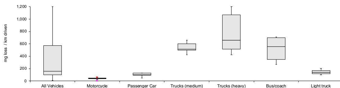
Figure 13-3: Loss rate reported in literature for tread loss of different types of vehicles
